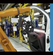
Part of the **MetraSCAN 3D R-Series**, the robot-mounted optical CMM 3D scanning system is a fast and accurate scanning solution designed for 3D automated inspection of parts on the production line and on the shop floor.
