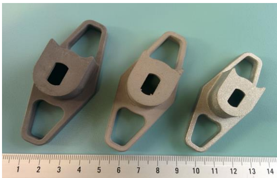
'Green', 'Brown' and Fired CP Titanium Parts Manufactured by PGE Injection Moulding Ltd., Hamilton.
